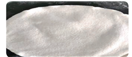
Add catalyst before adhesion, that is, the surface of the filter layer is clean without catalyst adhesion
