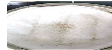
Adhesion of catalyst on the surface of filter layer after sample spraying by one-step dipping method
