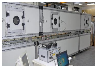
HVAC filter test
