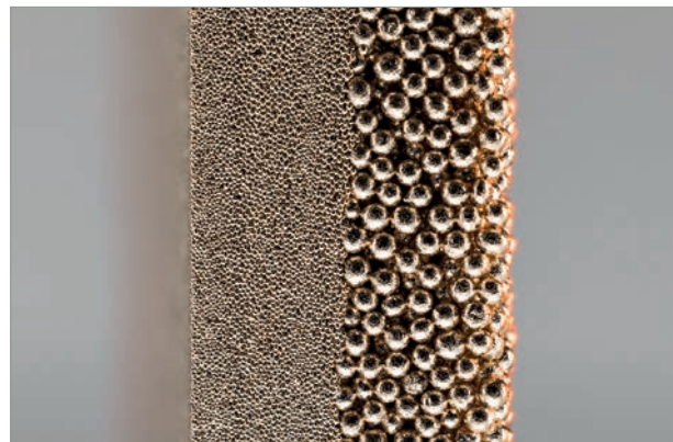
Bronze filters – SIPERM® B (Pore size 5 – 200 µm)
