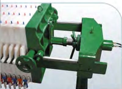
Double acting mechanical lock nut type Hydraulic Cylinder coupled with distance piece
