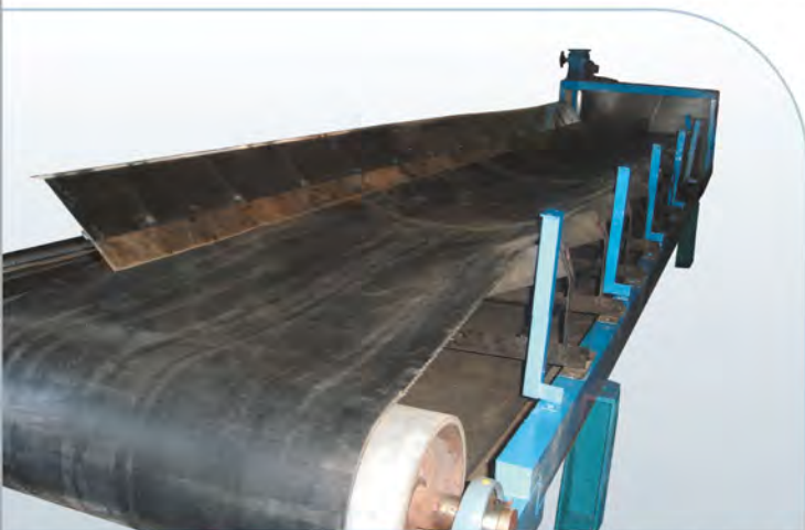
Rubber Belt Conveyor and Hopper Assembly.
