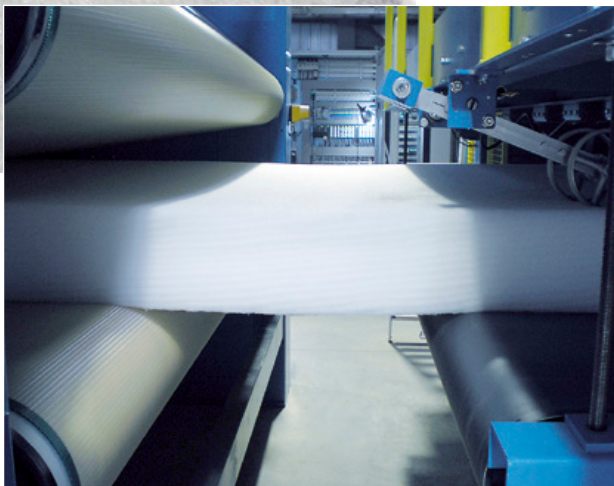
High temperature resistant belts in a thermal bonding application
