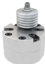
**Closed-loop Density Control** - The TruFlow Meter measures the actual material flow of solid and foamed adhesive. A PID control loop compares actual flow to the calculated pump rate and meters gas flow to achieve and maintain the gas/adhesive mix. Closed-loop density control is capable of density reduction to within +/-1.0 percent of the desired value.
