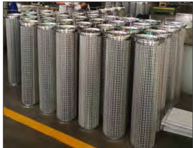
High capacity pleated filter element 1.0 m long
