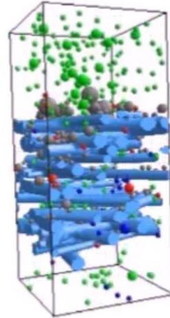
**Fig. 2:** 1-way coupled CFD-DEM simulation of the deposition of solid polydisperse particles at a nonwoven, showing particle adhesion and detachment at varying flow velocities. See the animation at <https://youtu.be/dO1Sz-KwiCA>
