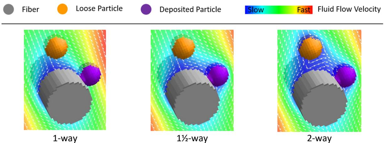
**Fig. 1:** Different CFD-DEM coupling approaches in DNSlab. With 1-way coupling, all particles don't affect the fluid flow. With 1½-way coupling, only deposited particles affect the fluid flow. With 2-way coupling, all particles affect the fluid flow.
