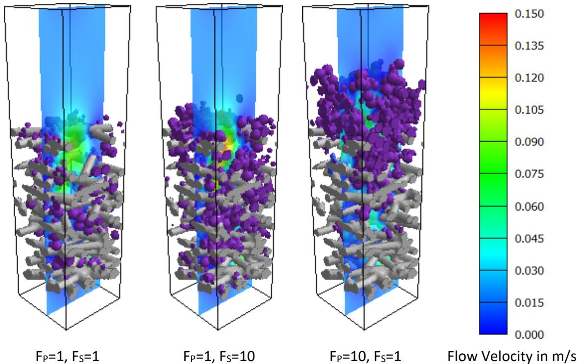
**Fig. 5:** Simulated distribution of deposited particles **after backwashing** (same units and color scale as in Fig. 4).
