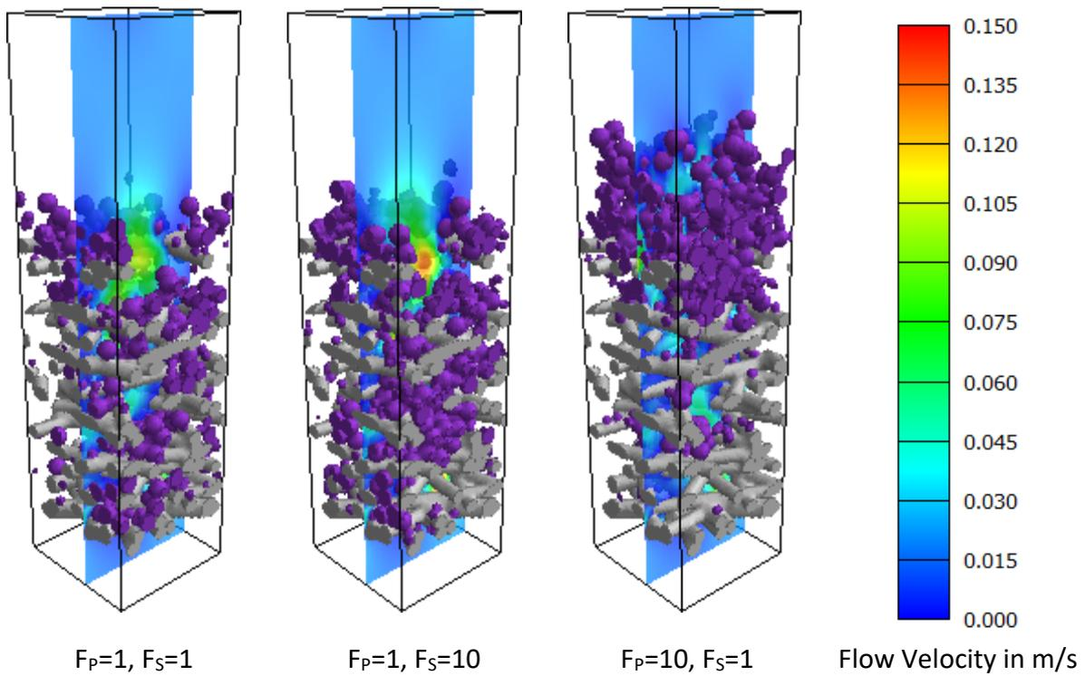
**Fig. 4:** Simulated distribution of deposited particles **before backwashing** for varied adhesion forces between particles and particles ( $F_p$ ) and between particles and fiber structure ( $F_s$ ). The adhesion forces are given in nN.
