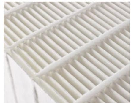
Filter production is characterised by a high material input; in fact, several kilograms of adhesive can be processed in a single filter.
