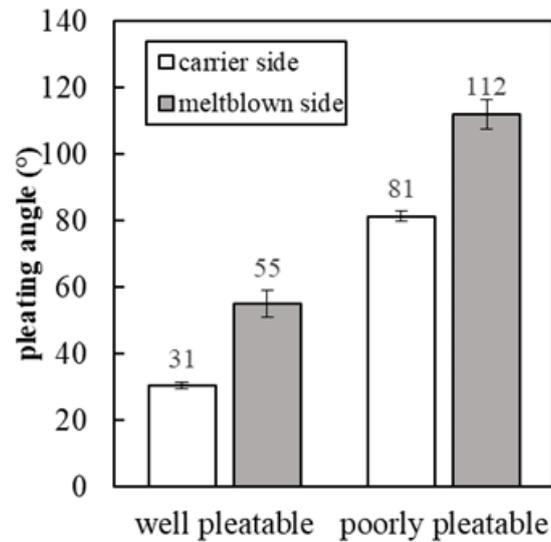
Fig. 4: Pleating angle of the well and poorly pleatable market samples, carrier side & meltblown side;  $n=12$ ; Error bars show the standard error of the mean  $SEM = \frac{s}{\sqrt{n}}$
