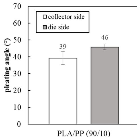
Fig. 6: Pleating angle of the PLA/PP blend, collector side & die side; n=12; Error bars show the *SEM*
