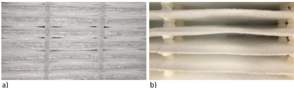
Fig. 1: Synthetic PP based filter panels based on a) rotative- and b) blade pleating.
