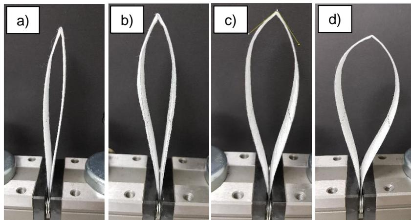
Fig. 3: Pleating angle of media 1 a) spunbond side, b) meltblown side; pleating angle of media 2 c) spunlaid side (yellow lines for analyzing the angle), d) meltblown side
