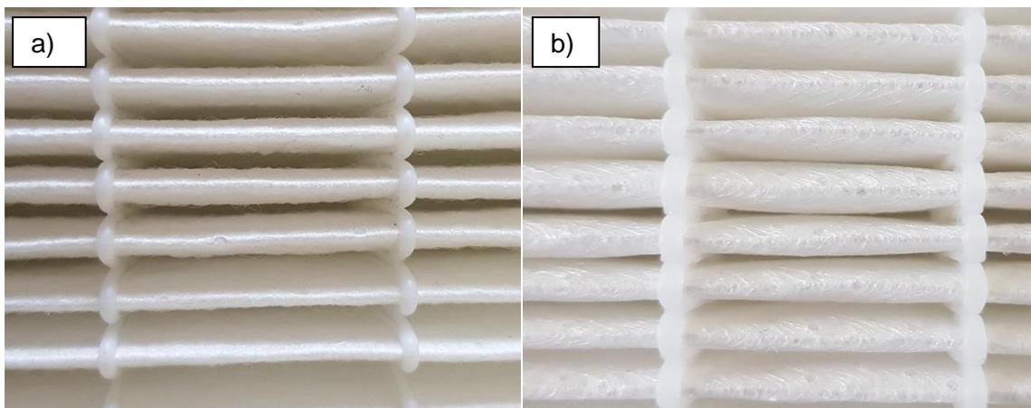
Fig. 5: View on the pleated filter element of a) medium 1 and b) medium 2
