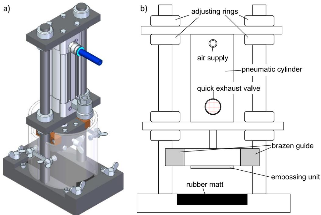
Fig. 2: Pleating device; a) 3D depiction, b) schematic figure
