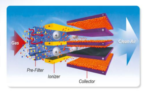
These charged particles then enter the collecting cell where oppositely charged plates collect the particles.
