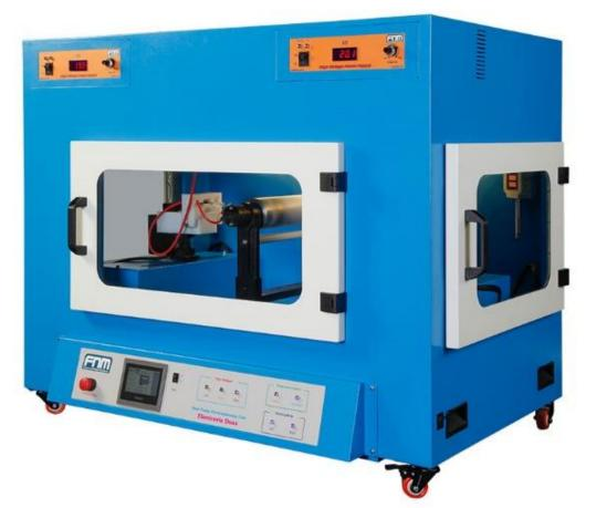
High voltage power supply Model: HV35P OV Max. output voltage: 35 kV Power: 35 watt Voltage monitoring: Digital, Accuracy: 0.1 kV Body: Durable metal casing Two high voltage power supplies are installed for dual pump series
