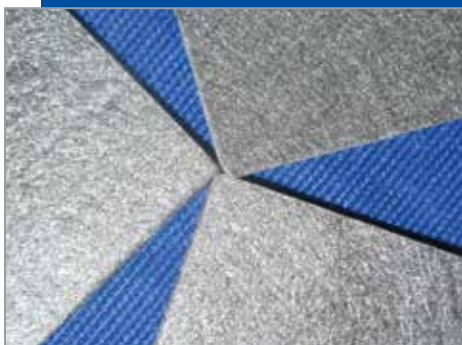
Sintered metal fiber felt Gesintertes Metallfaservlies
