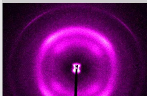
Fig. 1 2D diffraction pattern of coir fibre mounted in the TS 600 tensile stage while straining the sample.
