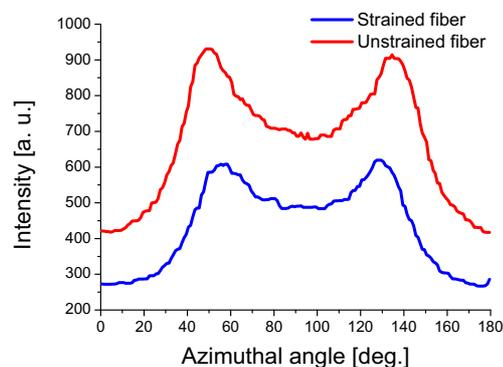
Fig. 2 Azimuthal integration along the 200 reflections. The position of the maximum is shifted to the center for the strained fiber.
