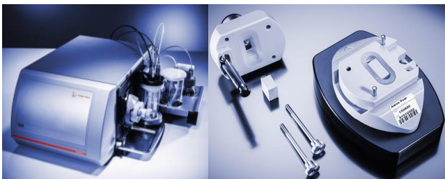
Figure 1: Left: SurPASS 3 equipped with dosing unit. Right: Adjustable Gap Cell with sample holders with a cross-section of 20 x 10 mm 2 .
