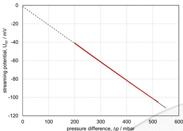
Figure 3: The zeta potential of a macroscopic solid surface is calculated from the slope of the linear dependence of streaming potential (or streaming current) on the differential pressure.
