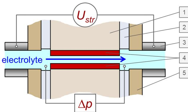
Figure 2: Schematic drawing of the Adjustable Gap Cell for planar samples (1 sample holder, 2 gasket, 3 electrode, 4 sample, 5 Adjustable Gap Cell)
