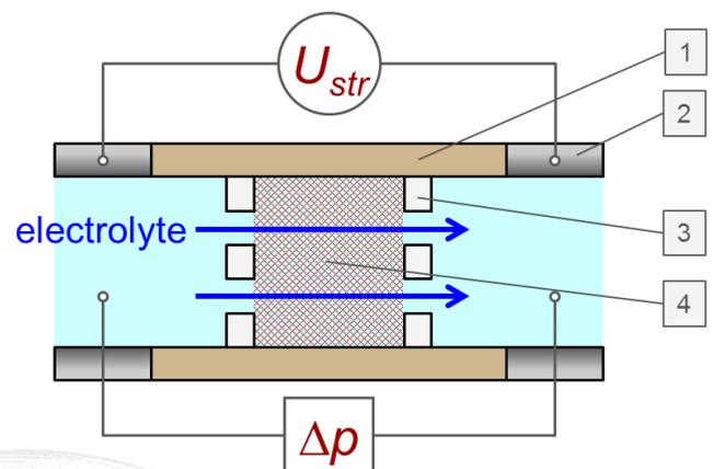
Figure 1: Schematic drawing of the Cylindrical Cell for fiber and powder samples (1 Cylindrical Cell, 2 electrode, 3 support disk, 4 sample plug)
