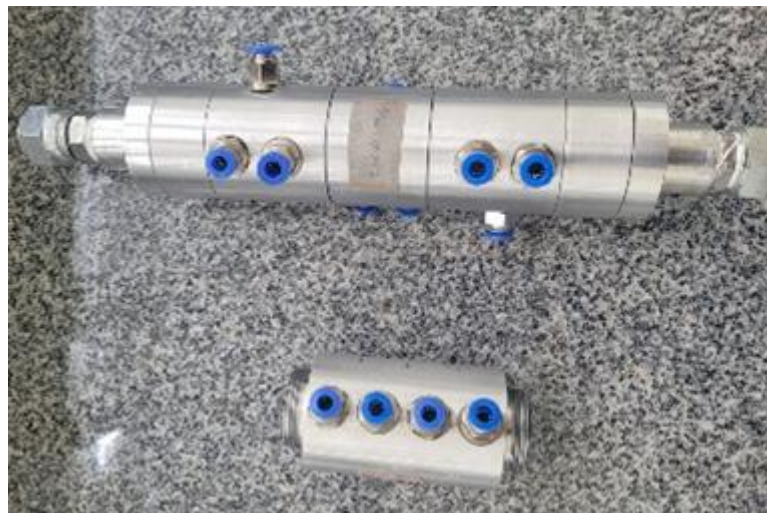
Figure 2 – Convergent-divergent nozzle and separator (Authors, 2026).
