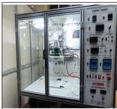
Figure 13: Electrospinning machine with facility of three-dimensional fibrous mat
