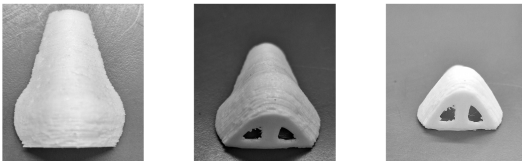
Figure 12. Actual 3D printed nose mask in different views
