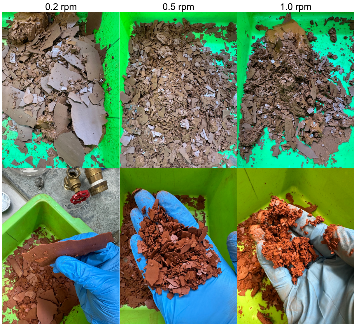
Figure 4: Pictures of red mud filter cakes produced by HPDR at average roller speeds of 0.2, 0.5, and 1 rpm, with a constant roller speed differential of 10% and hydraulic pressure of 68.8 \pm 1.7 bar. The corresponding cake solids concentrations were 70.0 \pm 1.3 , 67.4 \pm 0.6 , and 58.2 \pm 0.8 wt.%, respectively, demonstrating reduced dewatering performance with increasing roller speed.
