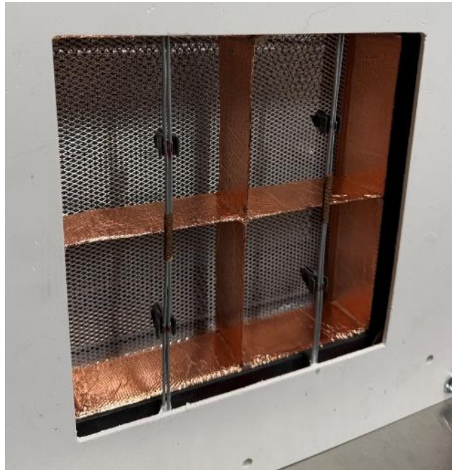
Figure 4: 2 x 2 Ioniser-array (4 brush ionisers)
